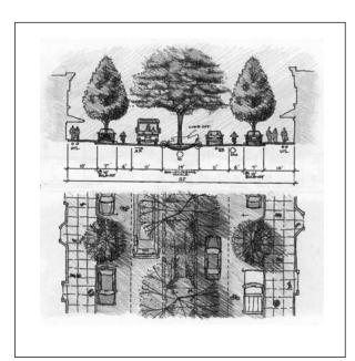
Figure 30—Trees can create a continuous canopy for maximum rainfall interception, even in commercial areas. In this example, a swale in the median filters runoff and provides ample space for large trees. Parking space-sized planters contain the soil volume required to grow healthy, large trees (from Metro 2002).
