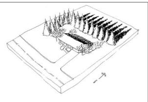
Figure 28—Mid-winter shadows from a well-located windbreak and shade trees do not block solar radiation on the south-facing wall (from Sand 1993).
